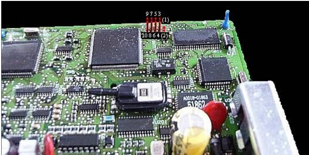
The BDM connector on the T7
